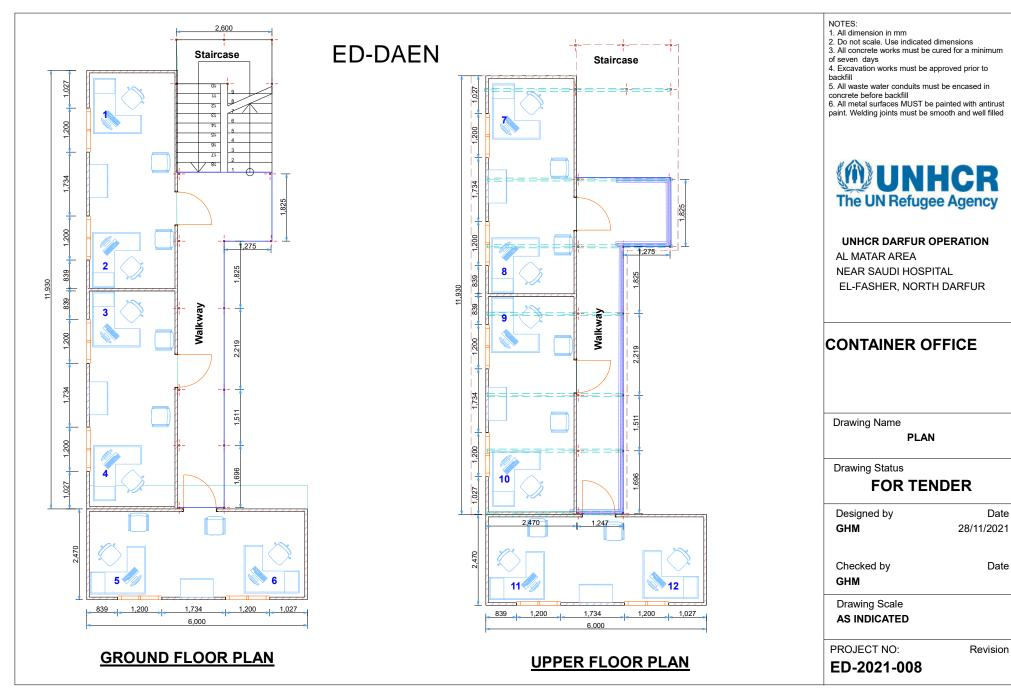
NOTES: 1. All dimension in mm 2. Do not scale. Use indicated dimensions 3. All concrete works must be cured for a minimum of seven days 4. Excavation works must be approved prior to backfill 5. All waste water conduits must be encased in concrete before backfill 6. All metal surfaces MUST be painted with antirust paint. Welding joints must be smooth and well filled
